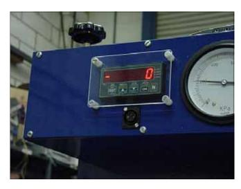
A digital display readout on the machine's front panel allows the operator to see the load currently being exerted, the operator can then use this display to more accurately set the required load for grading in Newton's instead of Kpa.
